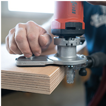
Even solid wood edges can be machined with commercially available cutters.
