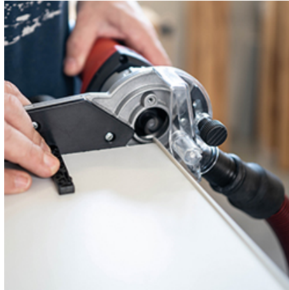
Plug-in fence serves as reliable guide when machining corners.
