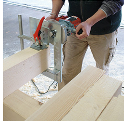
Speed: 8 to 18 mortise/tenon joints per hour.
