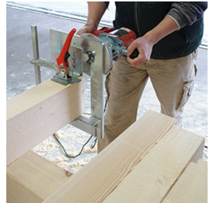
Speed: 8 to 18 mortise/tenon joints per hour.
