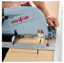
Attach the guide track to the long side of the opening. Cut the short side freehand, following a mark. Cut the long side by running the tip of the base plate along the guide track.
