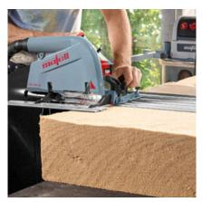
Flexible materials, as used to insulate the space between studs for example, can be cut quickly and accurately with the DSS 300 cc as well.
