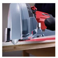
The MF-GF 90/15 cuts 90° V-grooves with very little dust; by gluing the cut faces, sturdy corner paneling is produced in just a few steps.
