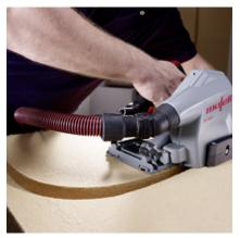
Service ducts can be cut in soft fiberboard quickly and without any dust with the MF-VN 25 expanding groove cutter.
