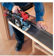
In combination with the roll-up Flexi-Guide FX 140, precise guided cuts up to 1.4 m (4.6 ft) long can be executed with consummate ease.
