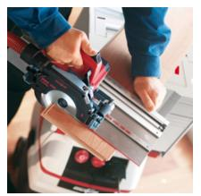
Fastening the portable circular saw to the KSS rail creates a very practical single-handed cross-cutting system.
