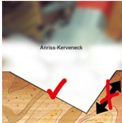
Unsurpassed precision – approved right-angled height adjustment. Distance of noches always constant irrespective of wood tolerances.
