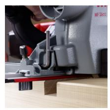
When cutting crosswise grooves, typically for risers or shelves, use of the guide 400 is recommended.
