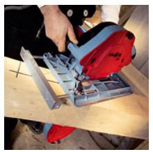
The efficient blower ensures a clear view of the mark.
