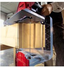
Thanks to high torque, solid wood and cutting depths up to 305 mm (12 in.) are not a problem for the Z 5 Ec.
