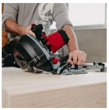
The NFU 50 can also be used as a skew notch and tenon cutter.
