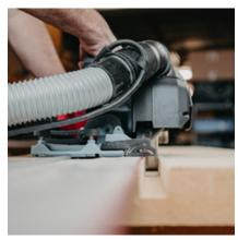
Grooves measuring 22 mm (7/8 in.) to 40 mm (1 9/16 in.) can be produced using the expanding groove cutter available as an optional accessory.
