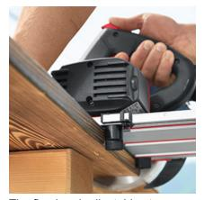
The fixed and adjustable stops on the underside of the rail allow the system to be used for angle cuts from +60° to -60°.
