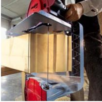
Thanks to high torque, solid wood and cutting depths up to 305 mm (12 in.) are not a problem for the Z 5 Ec.
