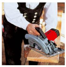
The angle can be set exactly and fixed on the scale between 0° and 45°
