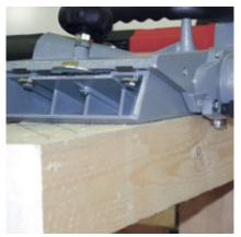
With guide rollers - for maximum utilisation of the planing width.
