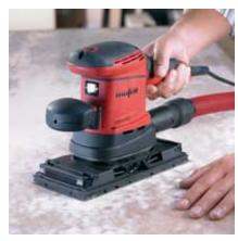
Very fine surfaces or high removal rates – in combination with the appropriate Abranet® abrasive mesh, the UVA is extremely versatile.
