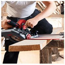
Thanks to the generously-sized angle scale, miter cuts can be realized that ensure a perfect fit.
