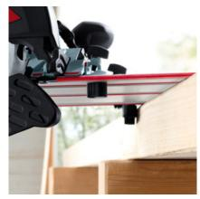
The fixed and adjustable stops on the underside of the rail allow the system to be used for angle cuts from  $+50^{\circ}$  to  $-60^{\circ}$ .
