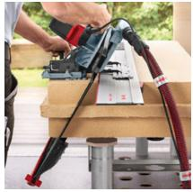
For exact bevel cuts, the DSS 300 cc can be continuously pivoted through 60° referencing the scale. To make the cut, use an auxiliary rest on or alongside the guide track.
