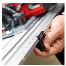
The highly graduated scale permits very precise angle setting.
