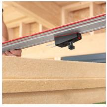
Insert a track clamp in both ends of the guide track, offer up the track and press the tips into the material. Attach the glider, offer up the DSS 300 cc, make the cut and the job's done.
