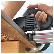
The fixed and adjustable stops on the underside of the rail allow the system to be used for angle cuts from  $+60^{\circ}$  to  $-60^{\circ}$ .
