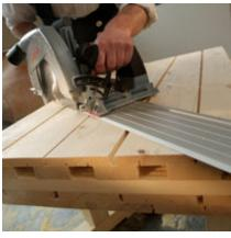
To enhance precision, the MKS 130 Ec can be used together with a guide rail.
