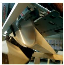
With a tilting range of 60°, the MKS 130 Ec is ideal for compound miter cuts. Even at this angle, the maximum cutting depth remains an impressive 65 mm (2 9/16 in.).
