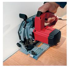
Perfect edging: the circular saw's spacers enable you easily to make exact expansion joint cuts with widths from 13 mm (1/2 in.).
