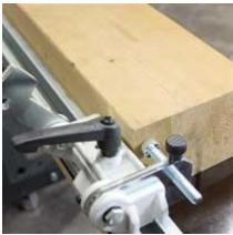
The 3 m (9.8 ft) long support profile with mm scale and length stop allows precise positioning of the workpieces.
