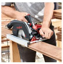
Using the MAFELL guide tracks or the parallel fence included in the delivery scope, which is graduated in millimeters, decking boards for instance can be made to fit exactly.
