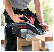
By retracting blade alongside the second handle, offering up the machine is easy and safe, especially when executing bevel cuts.
