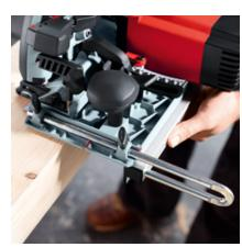
Working close to the edge is facilitated by the K 85-UA roller edge guide. Use the scale marked on the arm to set the spacing.
