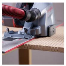
Three slots can be cut in one pass with the MF-SE 3. This quick and simple bending technique is applied to produce curved elements.
