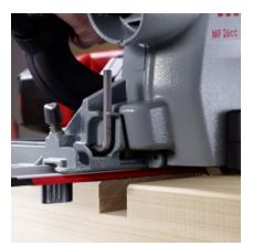
When cutting crosswise grooves, typically for risers or shelves, use of the guide 400 is recommended.
