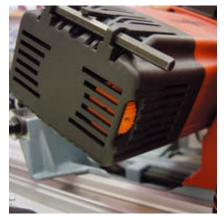
Setting wheel for speed adjustment for various materials.
