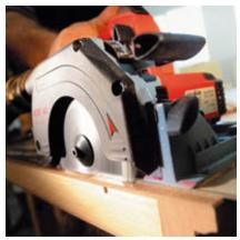
A handy machine combined with a guide rail ensure high precision, as shown when cutting doors to length.
