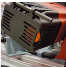
Setting wheel for speed adjustment for various materials.
