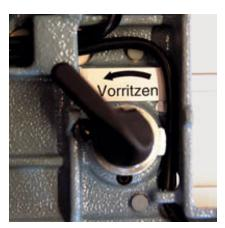
Saw unit can be set to scoring for tear-free cuts. Due to the scoring cut the cutting edge is shifted slightly.
