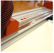
In conjunction with the integrated suction channel and the S 50 M, it eliminates practically all of the dust particles that occur.
