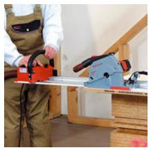
Due to the saw feed motor and convenient one-man operation panels can be cut easily and fast.
