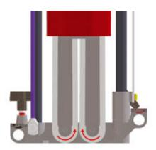
Two special mortising chains in opposite directions ensure tear-free work and optimum chip flow.
