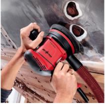
For coarse sanding, the EVA 150 E/5 is the ideal choice. The 5 mm stroke and a speed of 12,000 rpm represent the perfect combination for this kind of work.
